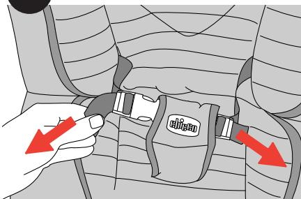
8B. Adjust the length of the waist belt to fit your child by pulling on the free ends as shown.
