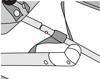
3B. Check to make sure the Back Rest Tube is securely attached, by making sure the buttons on the Back Rest Tube have popped into the holes on the tubes attached to the Base.
