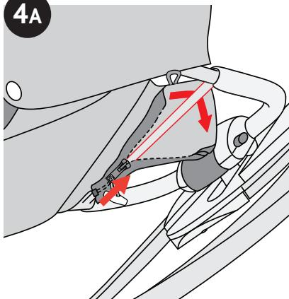
4A. Wrap the zippered end of the flap on the front of the seat around the cross brace tube as shown. Pull the zipper closed.
