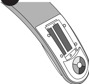
13B. Insert the new batteries; checking to make sure the polarity (+/-) on the batteries matches the markings on the product. Replace the battery cover and tighten screw.
