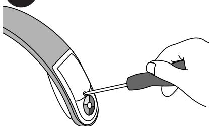
13A. This product uses (2) 1.5v AA batteries. To replace the batteries loosen the screw holding the battery cover with a Phillips screwdriver and remove the battery cover.
