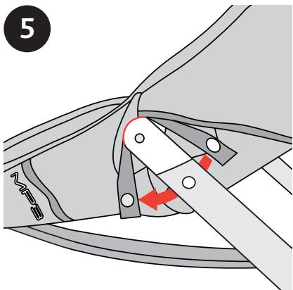
5. Position both straps on the side of the Seat to make sure that they go over the top of the seat frame tube as shown (in red). Wrap both straps down under the plastic hinge and snap together. Pull on the straps to make sure that the snaps are secured. Repeat step for the other side.
