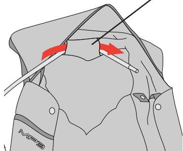
2B. Back Rest Tube as shown properly assembled to the loop on the back of the Seat.
