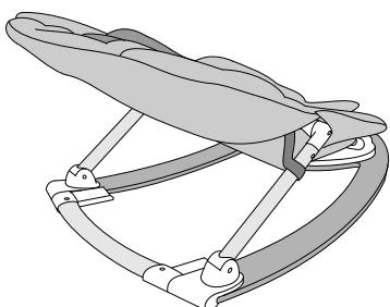
11A. Rocking Mode: Rear stand is rotated up and forward.
