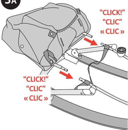
3A. Insert the ends of the Back Rest Tube into the front tubes attached to the Base. Press until you hear both sides click into place. Make sure the Seat is facing up after tubes are assembled.
