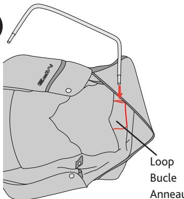
2A. Assemble the Back Rest Tube (D) to the Seat (B) by sliding the Back Rest Tube through a loop that is sewn at the top of the Seat under the flap on the back of the Seat.
