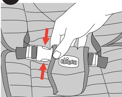
9. To unbuckle the waist belt pull back the crotch strap cover to expose the latch buttons. Squeeze both latch buttons together to release the waist belt. Repeat for other side.
