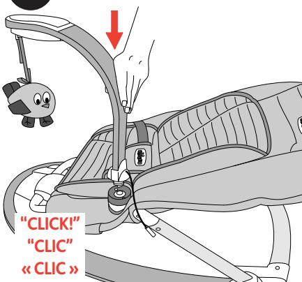
14. Hold the Electronic Toy Bar (E) so that it is facing forward as shown. Insert the Electronic Toy Bar into the Toy Bar mount and push down firmly until the Electronic Toy Bar "clicks" into position. Note: When the MP3 player is not being used make sure that the cord is tucked into the MP3 storage pocket.
