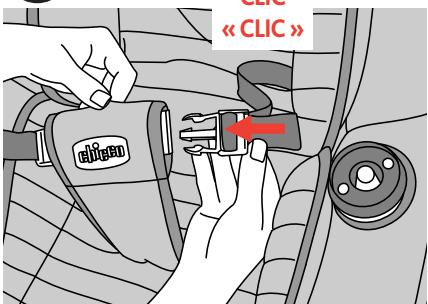
8A. To buckle the waist belt insert the ends of the waist belts into the crotch strap. Press until you hear a "click", pull on each waist belt to make sure it is properly latched into the crotch strap.
