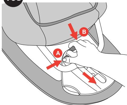
10B. To lower the seat: First press the release lock (A) and then squeeze the adjustment handle (B) on the sliding hub and move the hub forward.
