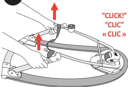
1. Open the Base (A) by pulling up on the rear legs. The frame is locked open when you hear a "click". Press down on the frame to make sure it is securely locked open.
